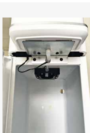
Fig. 6: Interior of the AQA drink Pro 20 cabinet without wastewater tank in place
